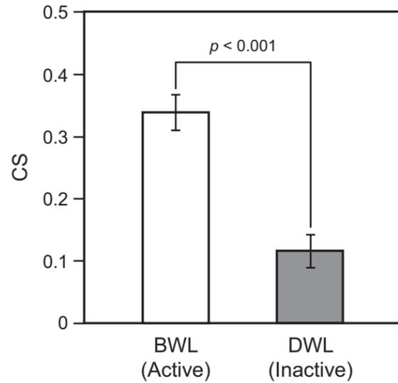
Mean CS values recorded by the bed Daysimeter when the lighting was programmed to be energized (7-10am). (The error bars represent standard deviation.)
