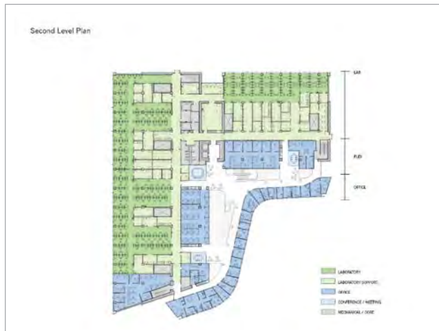
FIGURE 4: Typical lab floors of the Sandler Neurosciences Center are composed of an orthogonal, hyper-flexible lab block that supports a wide variety of possible lab configurations that can be tuned to the activities of individual researchers. Also included in this block is an innovative flex zone that can change between support offices or laboratory space.
