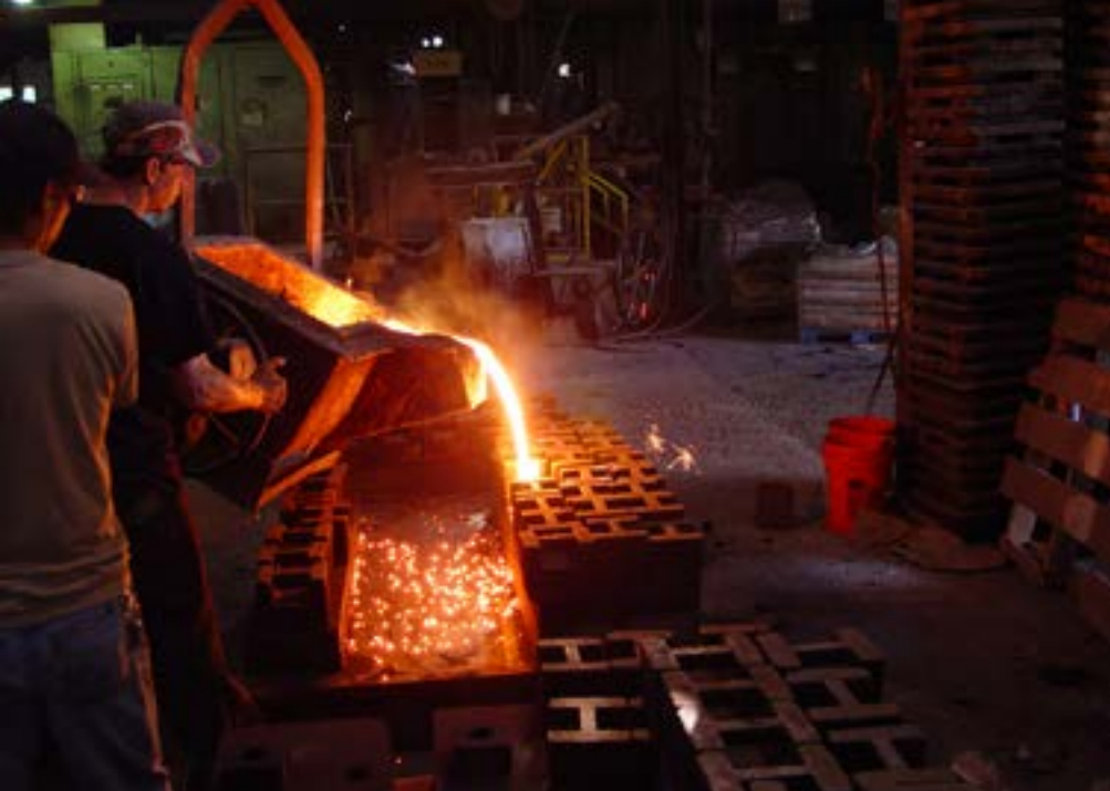
(PROCESS) Freshly cast balusters of cast iron created at Robinson Iron's foundry
