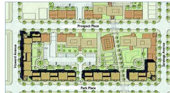
Rendered Site Plan, showing new Rental Apartments framing a shared landscaped Commons at block interior.
