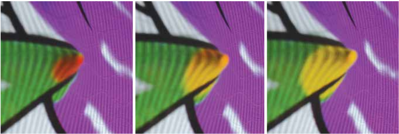
FIGURE 5. Size and color of the projection, at the point of interaction, changes from red to orange to yellow based upon the amount of pressure applied.
