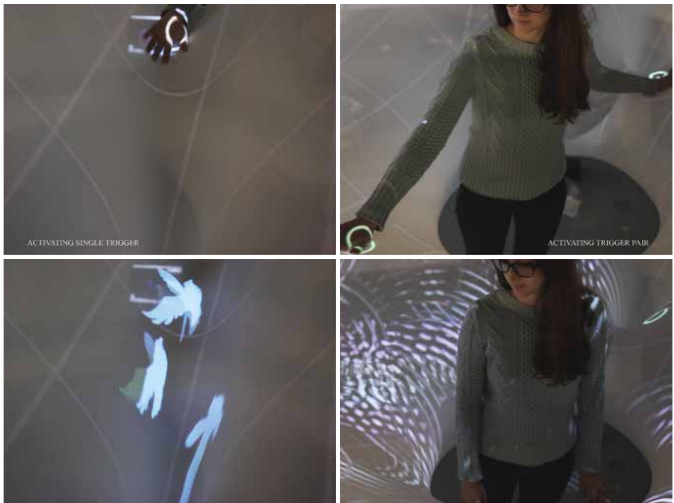
FIGURE 7. Animations and sound clips are played when the textile is depressed at certain locations. A pulsing circle is illuminated when a trigger found is found. Certain animations play by activating a single trigger,
