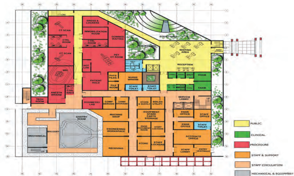
Figure 6: Second-floor plan: The entrance was designed at the same level as the imaging and support areas. A series of courtyards throughout the building balances the intimidating and sterile components with soft, sensitive elements. Evidence-based principles were adopted to create a design that reduces patient and staff stress and facilitates wayfinding.
