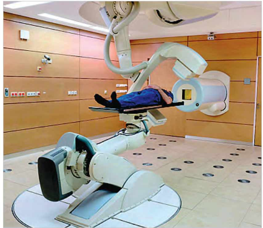
Figure 1: Siemens design of the patient table with the robotic arm for accurate positioning before treatment (retrieved from http://www.siemens.com on May 22, 2011)
