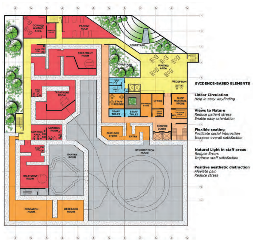
Figure 4: First-floor plan: Procedure and equipment areas were designed below ground level to use the earth around the building as a natural shield for radiation. The layout of the equipment room was based on the latest concept of locating the ion source and the linear accelerator within the circumference of the synchrotron ring, thereby decreasing the amount of space required. A horizontal beam treatment room, an angular room, and one with a gantry were designed to illustrate different room types.
